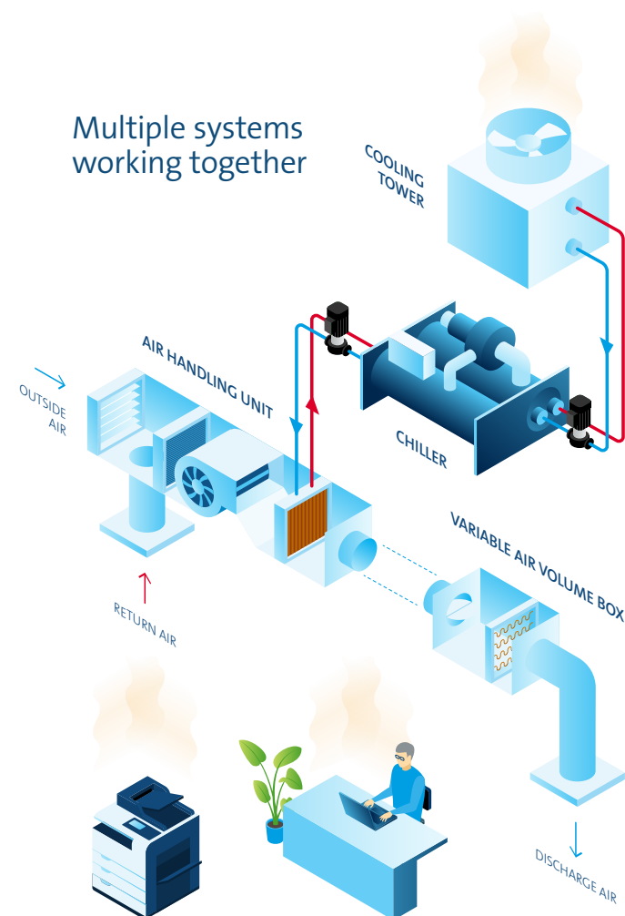
Figure 1.2 The figure shows how the water side (chillers, pumps and cooling towers) is connected to the air side (air handling unit and variable air volume box).
